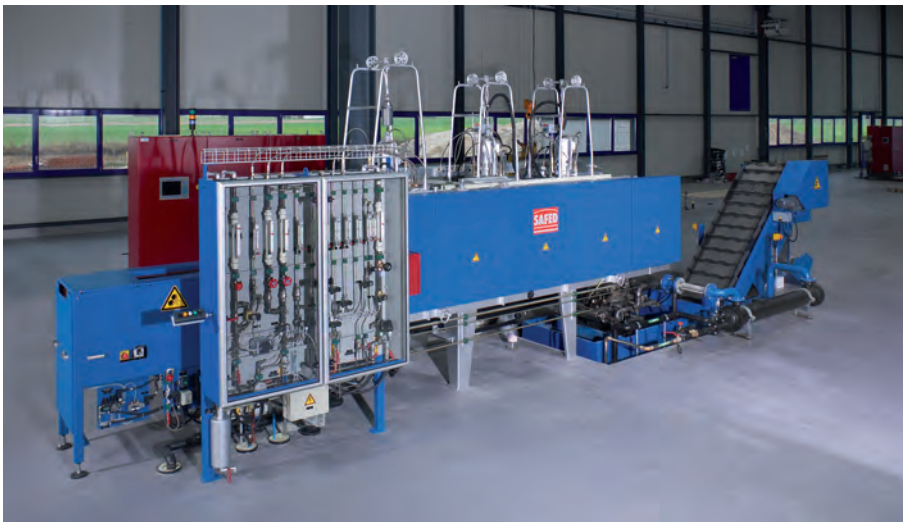
Fig. 4: Conveyor belt furnace for Oxycad NT® nitrocarburizing (Safed)
