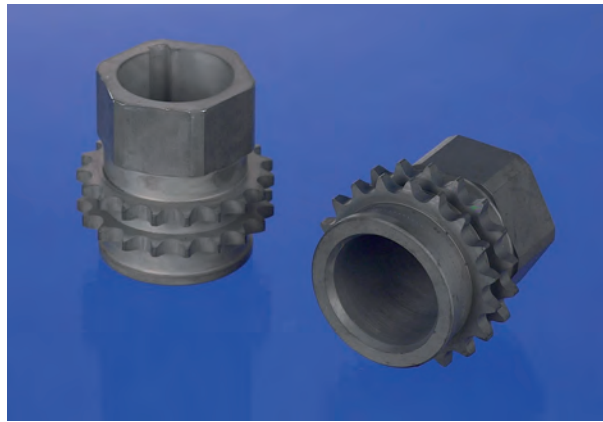
Fig. 7: Drive pinion for camshaft, 1.7131, 16MnCr5, nitrocarburizing (OXYCAD®)
